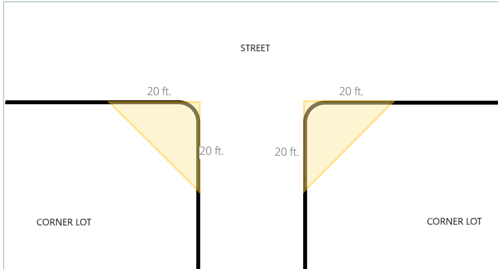
Figure 6: Diagram showing the Vision Clearance Triangle for corner lots
