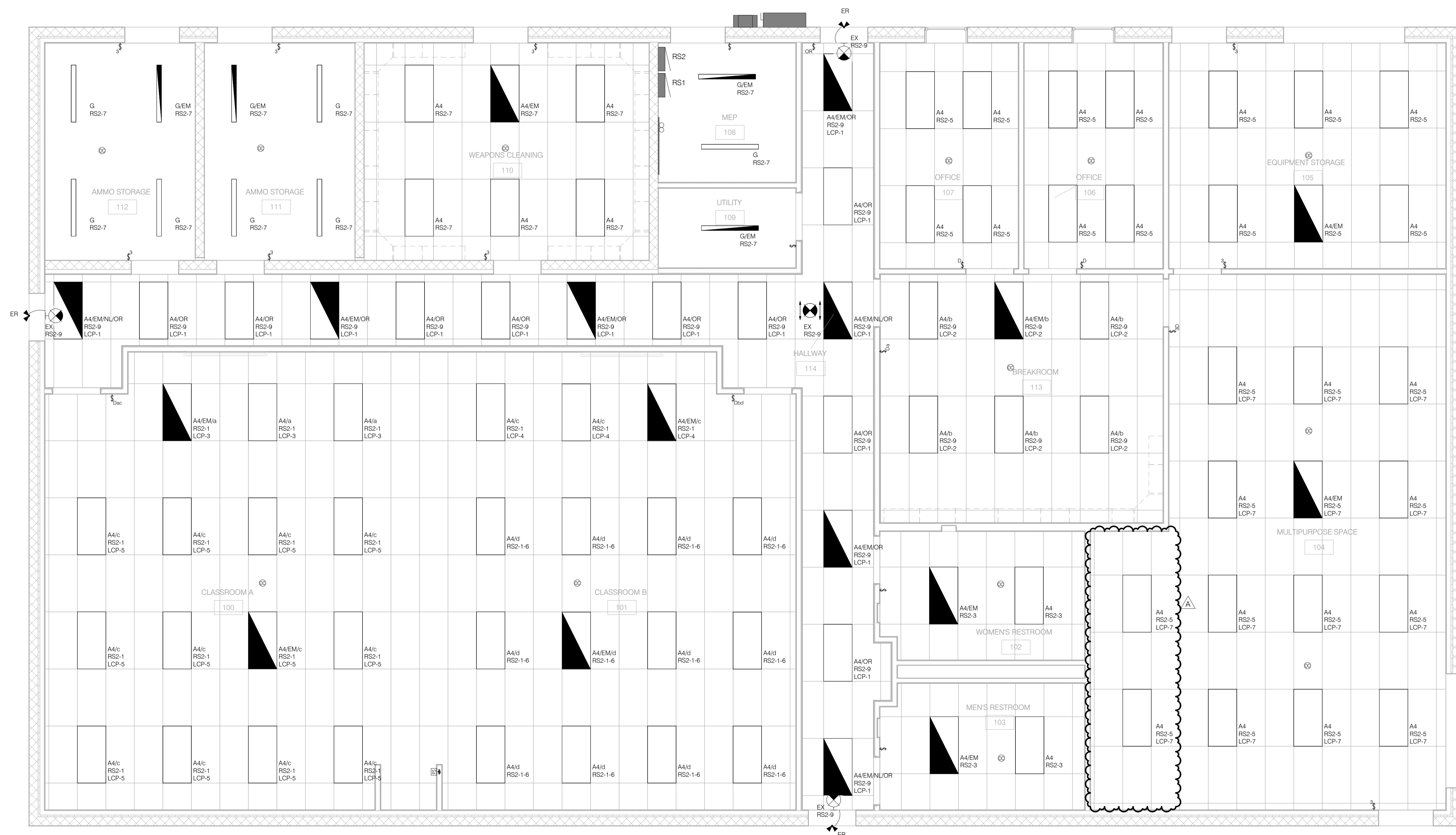
1 Range Support Building Lighting Plan 1/4" = 1'-0"
